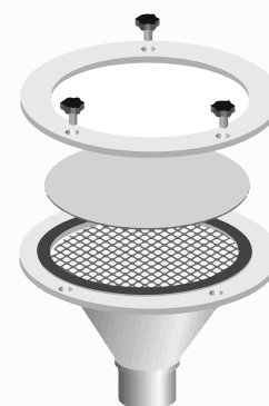
Filter holder for TSP collection detail
