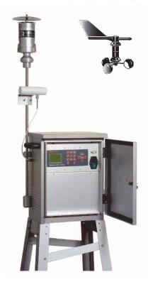
ECHO PM is a "stand alone" instrument projected also for outdoor operation in harsh climatic conditions. The wide regulation range and the accurate electronic flow sampling control at either actual or standard conditions, makes ECHO PM in accordance with the reference methods EN 12341 for PM 10 with head LVS PM10 2.3 m3/h, and US EPA 40 CFR part 50 for PMIO and PM2.5 at Im3/h.
